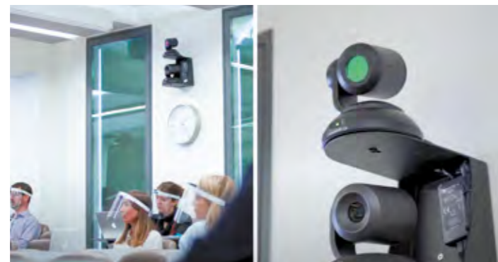
Hult's Limitless Learning technology uses intelligent speaker-tracking cameras, 360° ceiling microphones, and interactive virtual classrooms.
